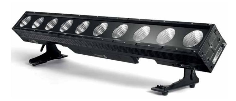
The CLF LEDbar PRO is a multifunctional linear LED batten. Because of the 24° beam angle it can be used as cyclorama as well as pixel controlled effect machine. 10 Big, individually controllable, high power RGBW LEDs deliver a rich color set and smooth HD dimming. Dynamic effects are easily configured by DMX, but the CLF LEDbar PRO is also Art-Net and sACN ready.
