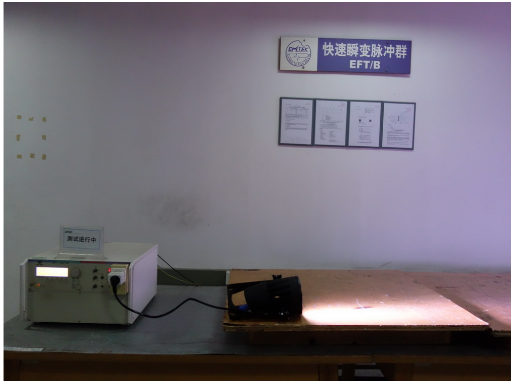
15.7 Photo of Electrical Fast Transient /Burst Test
