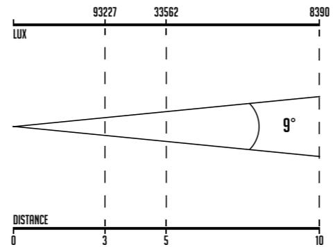
Designed for car shows and exhibitions or any other large scale venue, the Spectrum P1 Daylight is equipped with 36 high performance LEDs. Impressive output and a punchy 9° beam angle are ideal ingredients for long throw projection. Specially selected CREE LEDs provide a color temperature of 5700K at high CRI levels. 16bit dimming and flicker-free operation are also part of the feature set.
